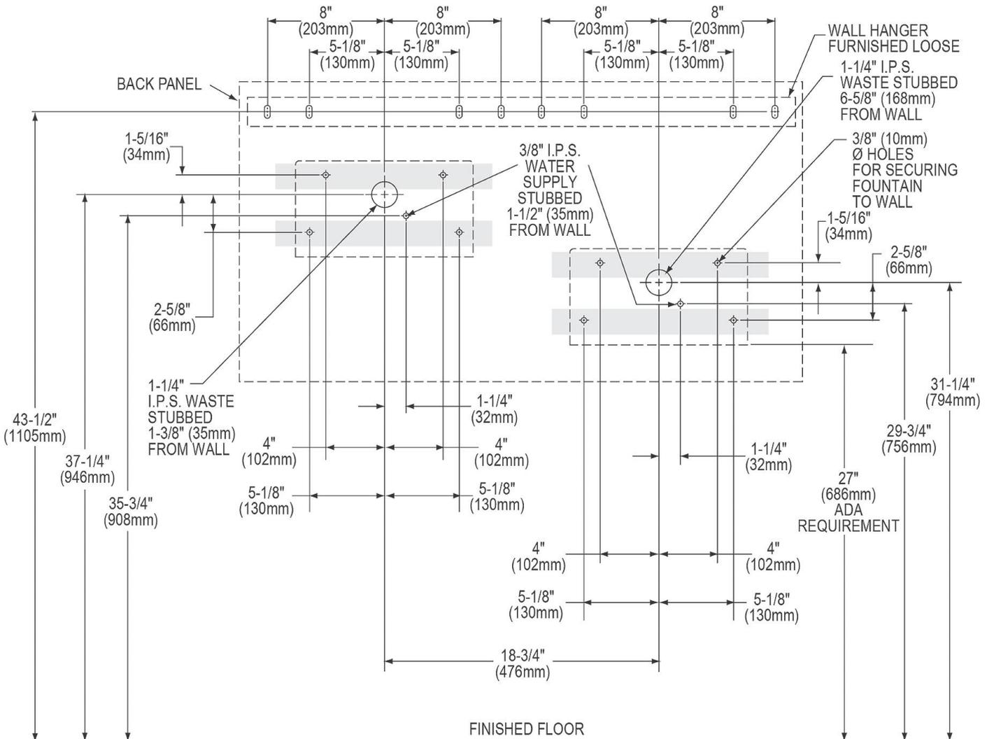
**NOTE:** When using MP20 Surface Mounting Plate, remove the wall hanger and back panel channels. See separate specification sheet for details on MP20 Surface Mounting Plate.
